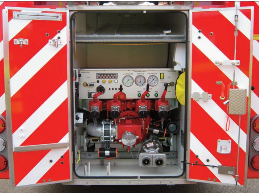
Above: pump bay on a MAN fire unit Below, right: hybrid configuration for Ashwoods' diesel-electric Ford Transit van
